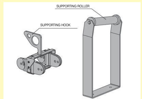
The chains from the "ROBOT" series are self-supporting and they do not need any support up to 200°. For applications with rotations exceeding that value it is necessary to use its own appropriate accessories. To reduce the problems of taking up too much space which generally is the case with the supports, especially on robots, Brevetti Stendalto has developed a series of supports which are capable of solving the problem.
