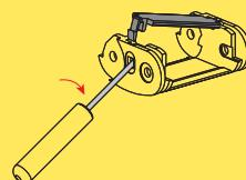
Special tool to remove the connecting pivots:
