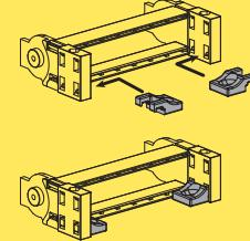
Reducers mounted on the outer radius
