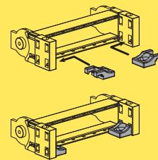
Reducers mounted on the outer radius
