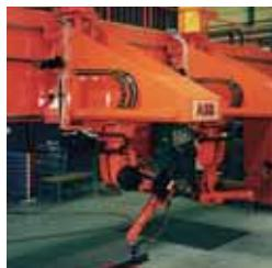
*Welding robot equipped with nylon chains.*
