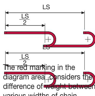
For applications with  $\frac{LS}{2}$  and weights not included in the area of the diagram showing self-supporting capacity, verify the possible use of support rollers (see page 30).
