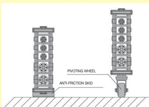
To make the movement easier and to reduce any friction on the cable chain, special changeable anti-friction skids or pivoting wheels have been designed.
