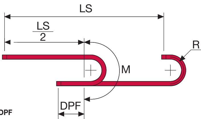
The chain length (**L**) is calculated by summarising the half stroke  $\frac{LS}{2}$  to the nominal value (**M**) of the bending radius and the distance (**DPF**) from fixed point to centre of total stroke.
