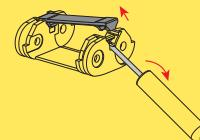
Special tool to remove the connecting pivots:
