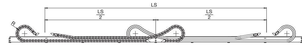
*A particular of the skid in the sliding of the chains in the Sliding series.*
