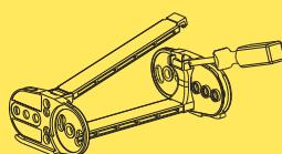
Special tool to remove the connecting pivots:
