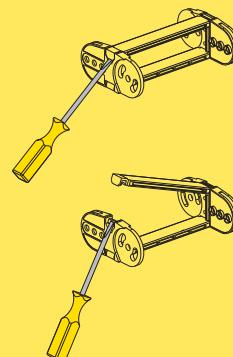
Special tool to remove the connecting pivots:
