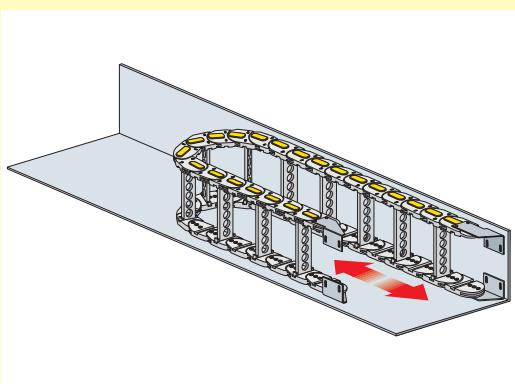
*Horizontal with chain mounted on its side
