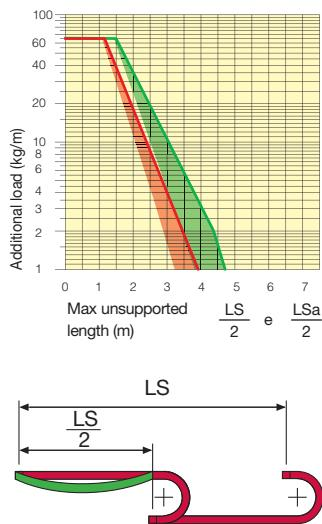
The area in the diagram considers the difference of weight between various widths of chain.
