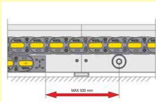
*Reduce as much as possible the distance between the fixed point of the cable chain and the starting point of the rollers or sliding plane.*
