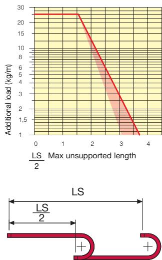
The red marking in the diagram area considers the difference of weight between various widths of chain.
