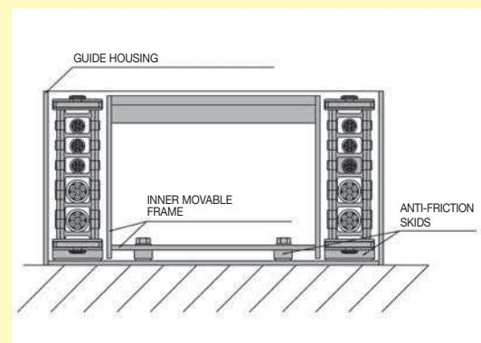
*To facilitate the sliding and reduce the friction of the cable chain, special changeable skids or pivoting wheels are taken into account.*
