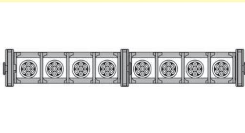
*Multiple side-band chains. If it was necessary to increase the self-supporting capacity and the stability when having a large number of cables.*
