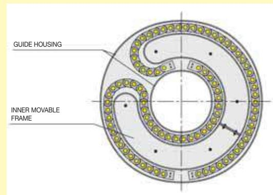
*For applications with rotations over 180° it is necessary to use two cable chains. For a correct usage they should be guided both internally and externally. A special inner movable frame, mounted on anti-friction skids or pivoting wheels in combination to the guide housing guarantees the rotation.*
