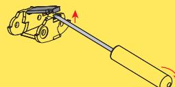
Special tool to remove the connecting pivots:
