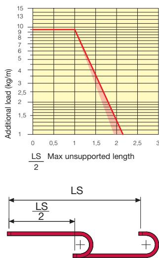
The red marking in the diagram area considers the difference of weight between various widths of chain.
