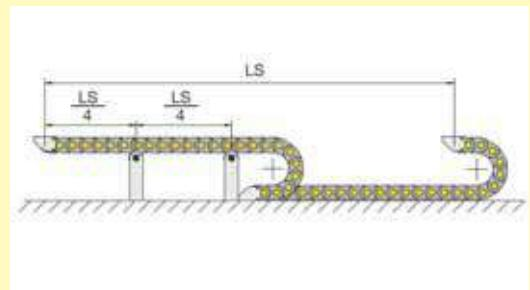
The length  $\frac{LS}{4}$  is included in the values of the diagram showing self-supporting capacity.
