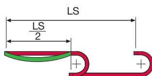
\*If the chain is in the ADMISSIBLE SAGGING area (between GREEN and RED area) version with frames on every link is necessary.
