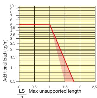
The red marking in the diagram area considers the difference of weight between various widths of chain.
