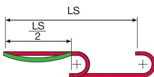
The area in the diagram considers the difference of weight between various widths of chain with nylon frame every second link.
