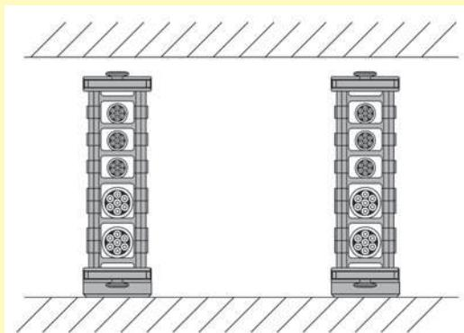
This kind of mounting becomes necessary when there is a limited space upwards and mounting the chain normally would take up too much space.
