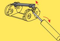
Special tool to remove the connecting pivots:
