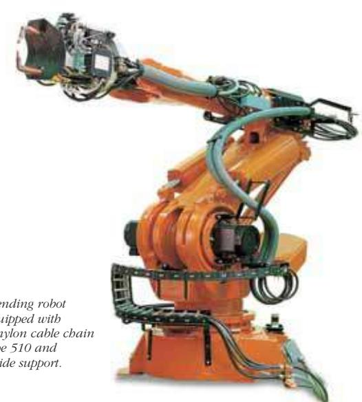
*Wending robot equipped with a nylon cable chain type 510 and guide support.*
