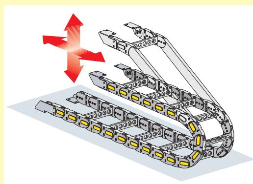
Combination of both vertical and horizontal movement.
