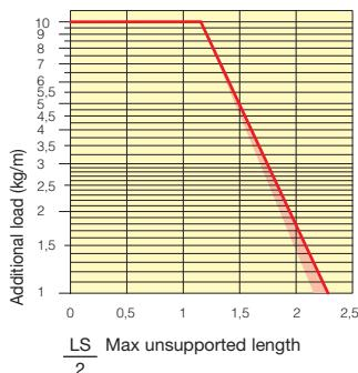
The red marking in the diagram area considers the difference of weight between various widths of chain.
