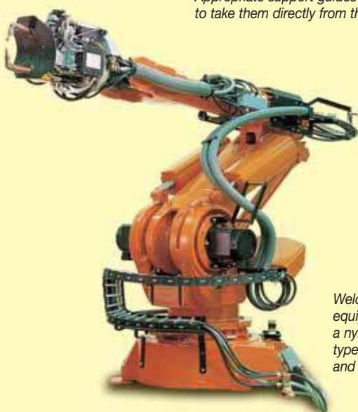
Welding robot equipped with a nylon cable chain type 510 and guide support.
