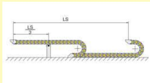
The length  $\frac{LS}{3}$  is included in the values of the diagram showing self-supporting capacity.
