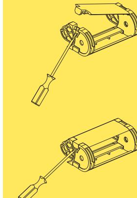
*Special tool to remove the connecting pivots:
