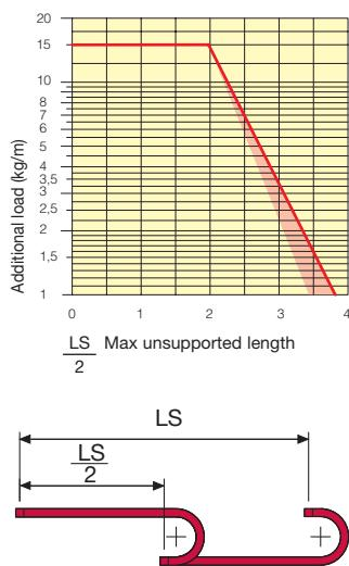
The red marking in the diagram area considers the difference of weight between various widths of chains assembled with nylon frames every second pitch.
