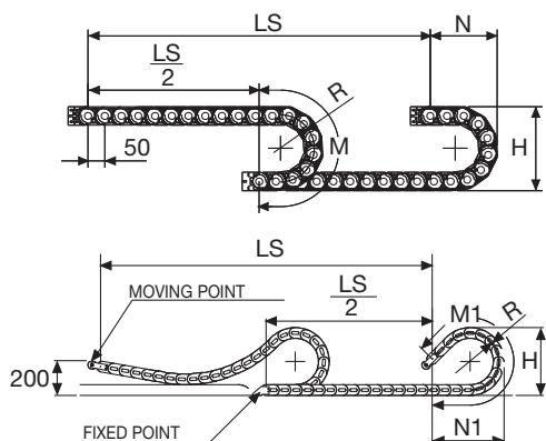
For sliding applications, technical data can slightly change according to frequency, added weight and environment.
