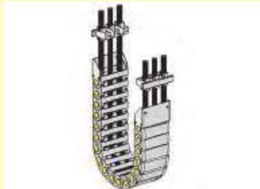
The placement of the cable/hoses is very important to ensure the application works properly. Cables/hoses have to be fixed at both ends using the appropriate accessories so as not to make their weight disturb the cable chain. In this type of application the cable chain should only guide the cables/hoses during their movement.
