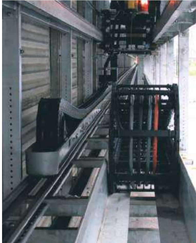
Chain testing rig for long travel: Tests at 8 m/s for 130 m travels.
