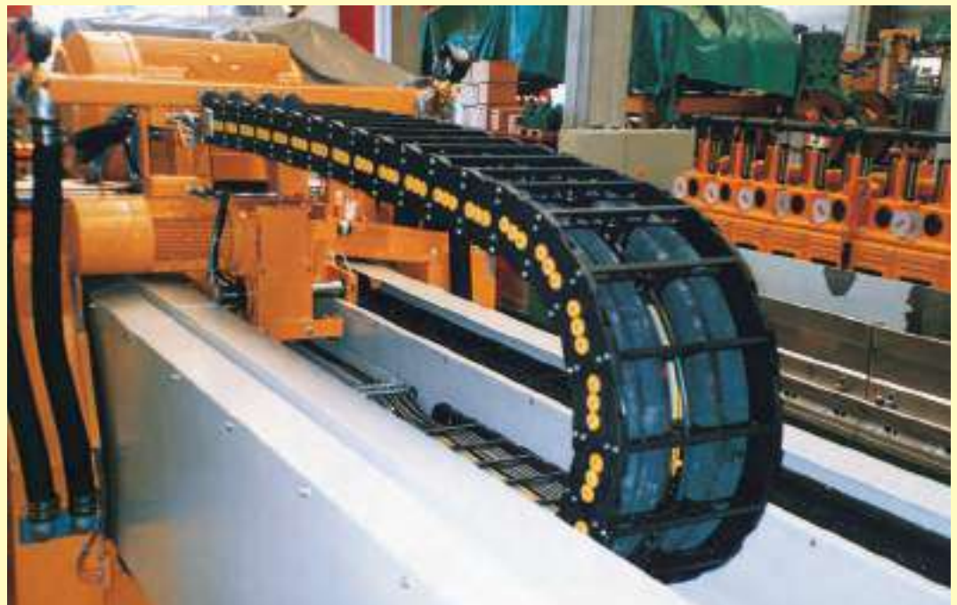
Nylon chain, type 310, in a self-supporting state.
