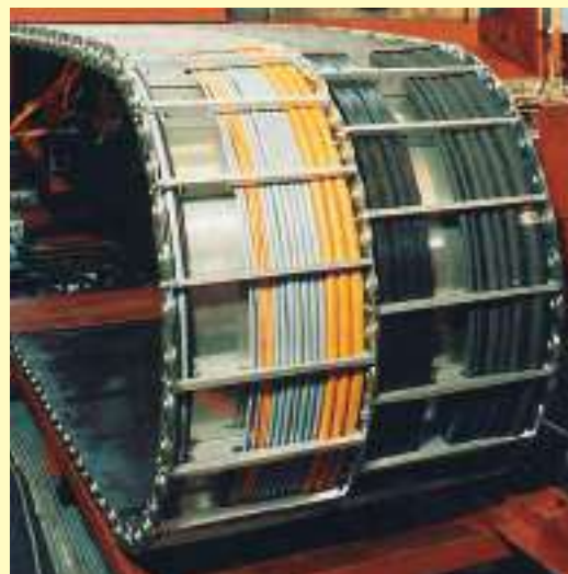
A 30 chain in steel with three bands and separations between electric cables and hydraulic hoses..
