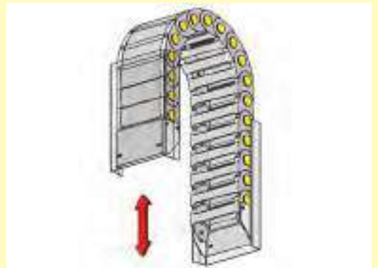
When applying the cable chain in this way some support is needed to avoid the chain to unbalance itself outwardly. Generally the cable chain must be supported both on the fixed and mobile points.
