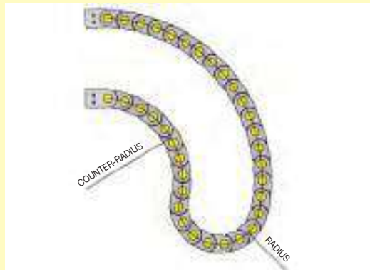
With the use of counter-radius chains it is possible to create rotations both on small and large equipment (e.g. parabolic antennas, rotating tables, cranes, telescopes).
