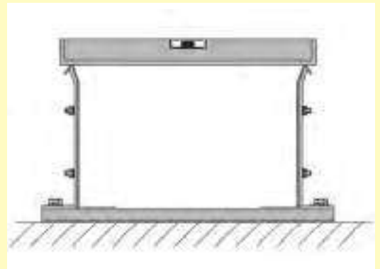
Verify that the plane on which the guide channel for sliding is mounted is perfectly aligned and smooth.
