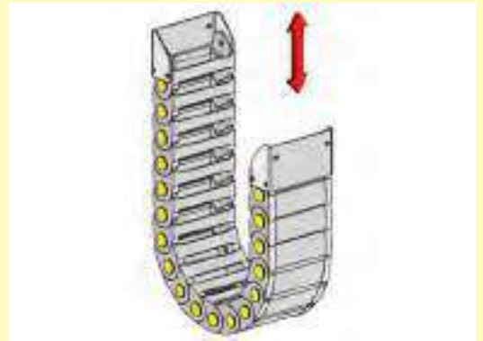
If the application only concerns one vertical movement the cable chain does not need any particular support.
