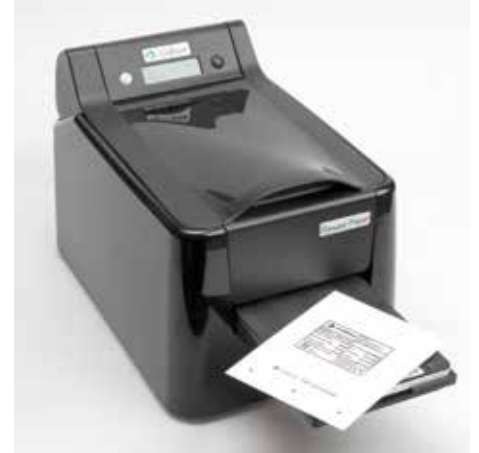
Recovering the card when printing is finished
