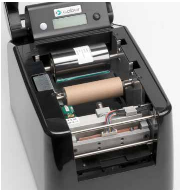
Inserting the ribbon
