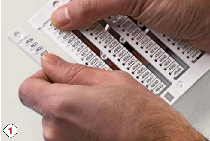
1 Remove the stem from the card.
