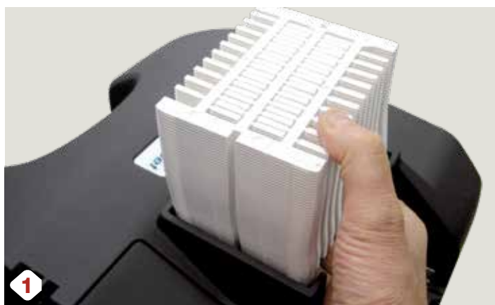
1 Insert the material in the feeder.
